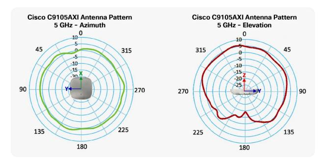
Figure 1. Antenna profiles
